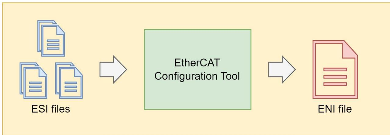
The EtherCAT Technology Group specifies that the EtherCAT MDevice Software must support at least one of the following in the Network Configuration section: *Online Scanning* or *Reading ENI*. This library, however, supports both. In the case of *Reading ENI*, this library currently extracts only partial information from the ENI file for network configuration.
