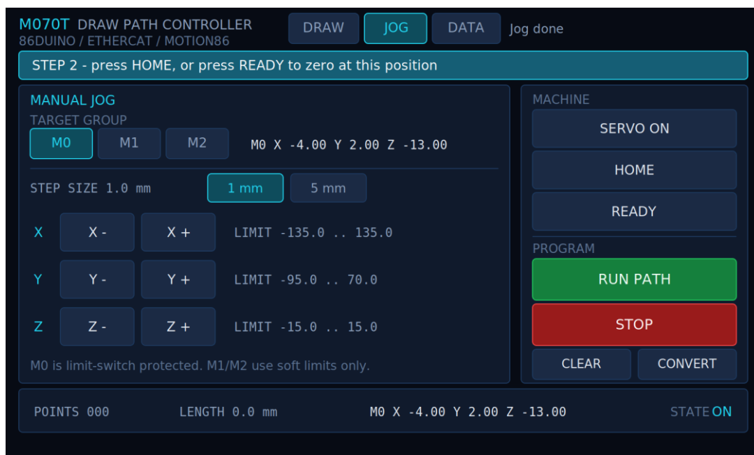
Figure 2 Jog page: machine group selector, step size, plus/minus buttons for X, Y and Z with their travel limits
